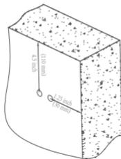
2. For stone, brick and drywall, insert a wall anchor (included) into each hole. Do not use wall anchors if wall is not stone, brick, or drywall. Screw the longer screw into the existing holes or wall anchors. Leave each screw exposed 0.21 inch / 5.0mm out from the wall.
